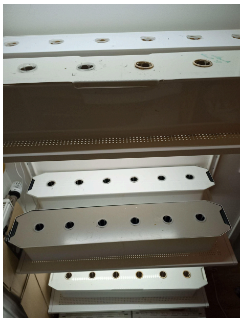
Figure 4: Experimental set-up showing the DWC experiment with the empty Harvy prototypes, prior to adding the water and seedlings. Post-experiment photo taken on 2024-06-18.
