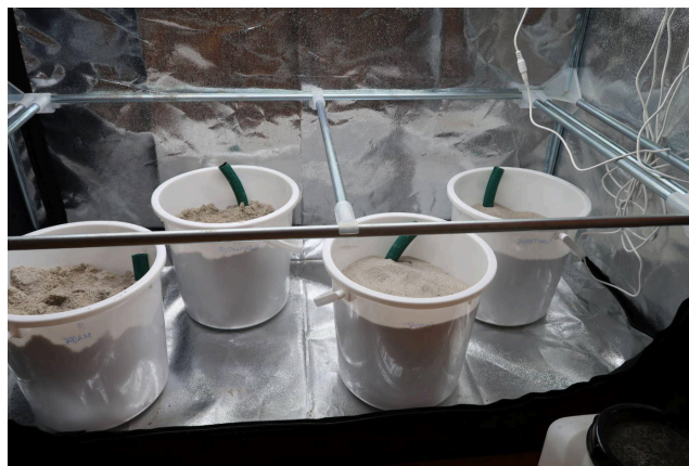
Figure 2: Experimental set-up showing the Media Bed experiment with the buckets, sand, and hoses. Note that only the two buckets closest to the camera were used for the experiment. Photo taken on 2023-06-28.
